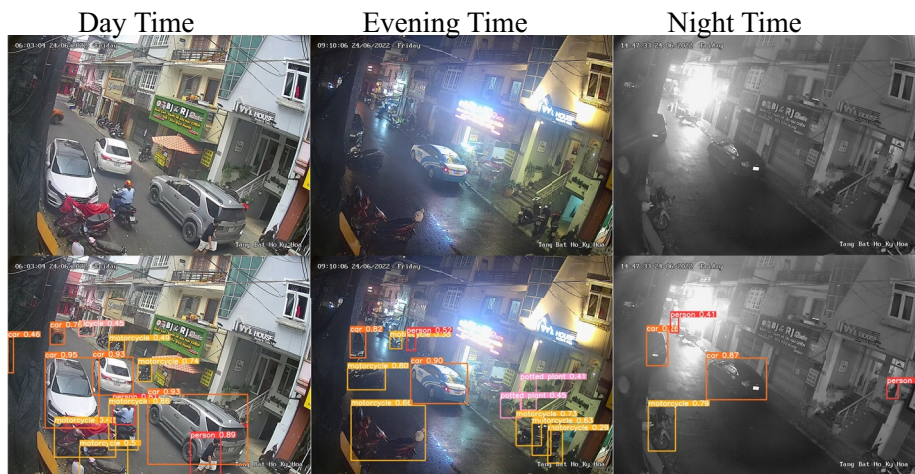
Figure 4. YOLOv8x weights used with the COCO dataset 26 to detect cars, motorbikes, and buses (labels used from the COCO dataset) 7 in the CCTV images 7 . Vehicle count from this detection is used for the discovery of Periodic traffic pollution patterns.
